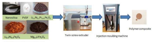
Materials used in the preparation of polymer composite
